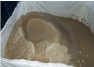
Draining then drying the struvite produced using a filter bag during tests at the Braunschweig WWTP in Germany, with phosphorus elimination efficiency levels higher than 85%
