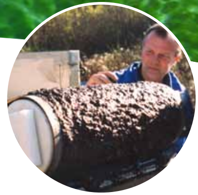
Concentrated sludge after filtration with the Hydrotech Beltfilter
