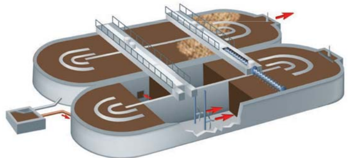
BIO-DENITRO with Oxidation Ditches
